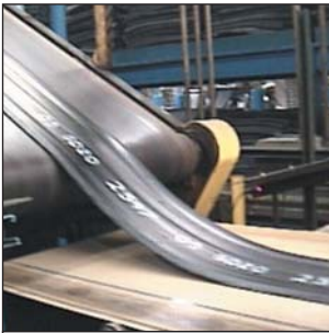
Extrusion Take Away Conveyor Recommend: uni SNB-M2
